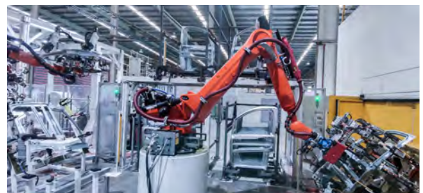
Vision-Guided Car Door Inner Panel Picking
