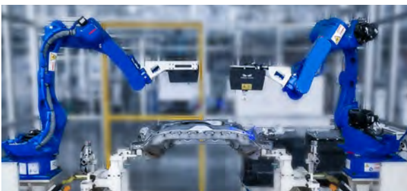
Subframe Inline Measurement
